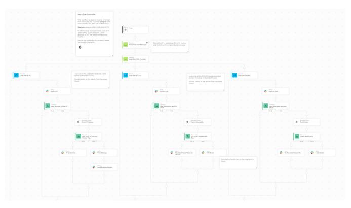
Example of a Torq workflow that enriches security events with Recorded Future intelligence data, communicating findings to security personnel handling the events over Slack.
